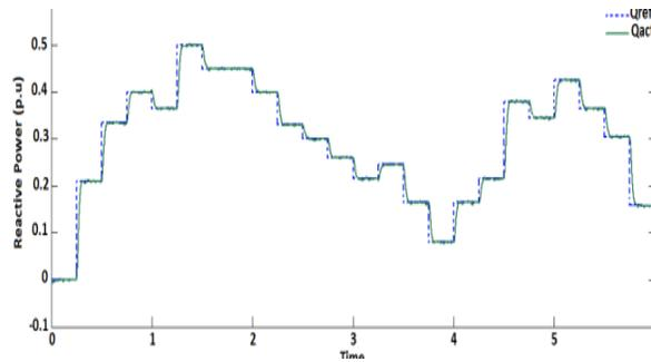
Figure 4 Tracking of reactive power demand of grid.
