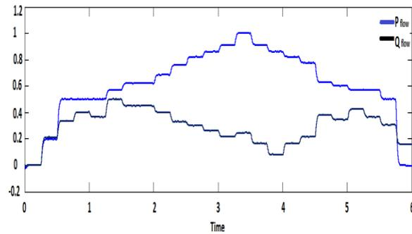
Figure 5 Independent flow of real and reactive power.
